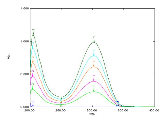
Fig.3: Zero order overlain spectra of Daclatasvir Dihydrochloride showing absorbance at 302nm.
