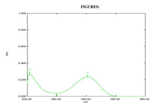
Fig.2: Zero order spectrum of Daclatasvir Dihydrochloride at 302nm.
