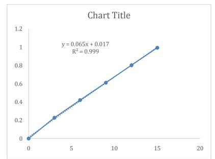
Fig.4: Calibration curve of Daclatasvir Dihydrochloride by zero order spectroscopy
